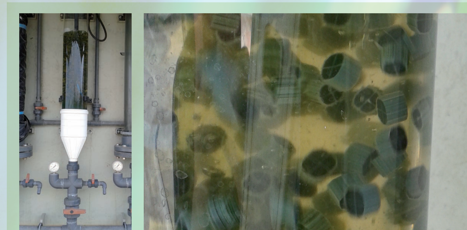
FIGURE 11. Photoreactor for outdoor microalgae cultivation.
